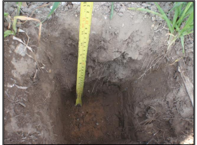
Plate 10 : Topsoil arisings from TH13 (agricultural soil)
