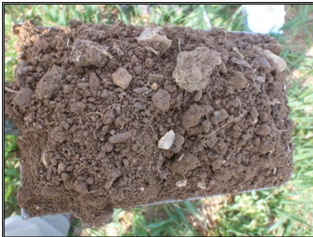
Plate 11: Topsoil arisings from TH13 (agricultural soil)
